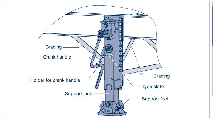
These BPW support jacks are intended for installing on a trailer vehicle. They provide support for the uncoupled trailer or semi-trailer, as well as for adjusting their height during the coupling procedure.
