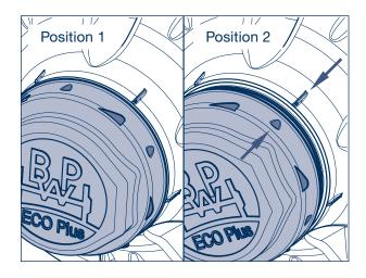
3. Tighten the axle bolt (WAF 46) using a hexagon socket spanner whilst simultaneously rotating the ECO hub unit.
