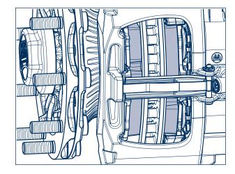
The brake pad thickness can be checked where the brake caliper meets the welded anchor plate with the wheels mounted (approximate wear indicator).
