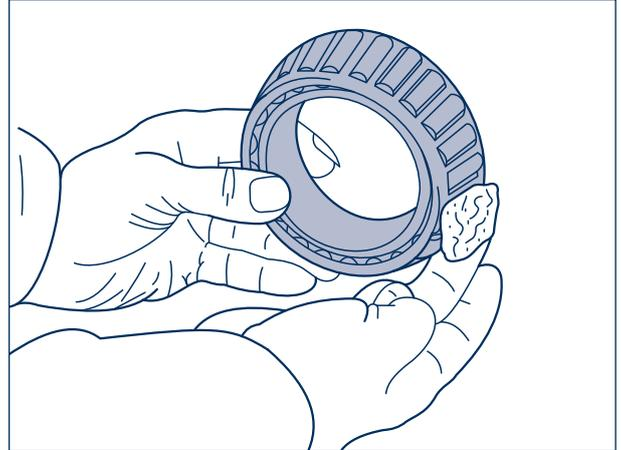
Clean wheel hubs thoroughly inside and outside. Clean taper bearings (using diesel oil) thoroughly, dry and check for re-useability. Replace seals.
